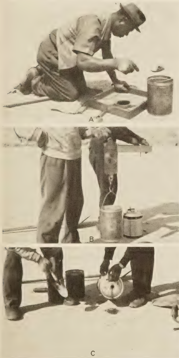
FIGURE 23.—THREE STEPS IN MAKING A DENSITY TEST: A, REMOVING LOOSENED BASE COURSE MATERIAL FROM HOLE; B, WEIGHING THE BASE COURSE MATERIAL REMOVED; and C, FILLING HOLE WITH OIL.
